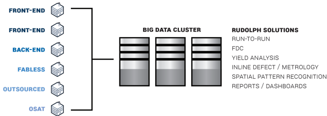
FIGURE 2. Numerous locations worldwide feed information into a single big-data cluster where multiple software solutions operate on the pre-aligned and internally consistent data set.
