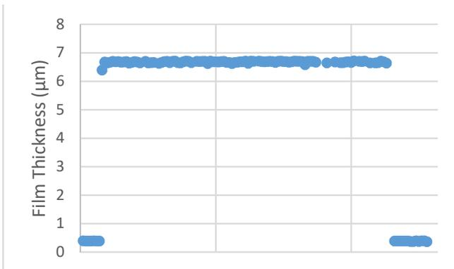
Figure 9. Film thickness profile of spray coated panel.
