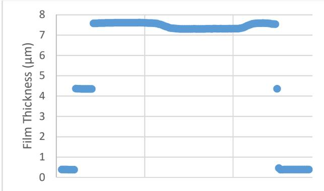
Figure 8. Film thickness profile of spin coated wafer.
