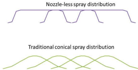
Figure 3. Spray distribution comparison between nozzle-less spray head compared to traditional spray nozzle.
