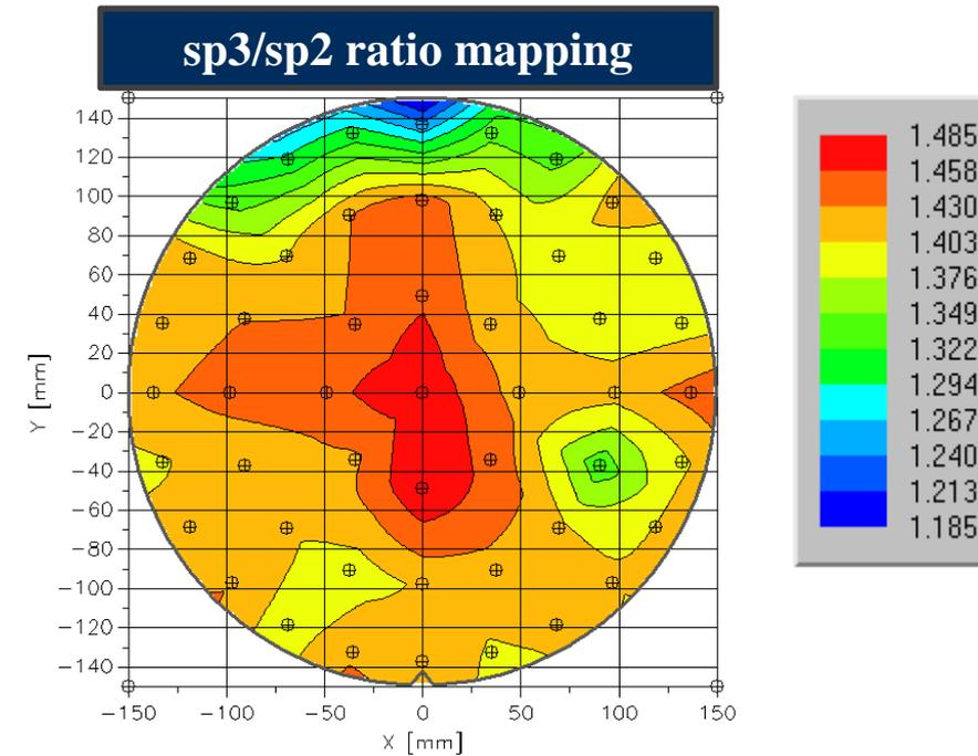
Characterization of the bonding structure of the materials using transmission FTIR
