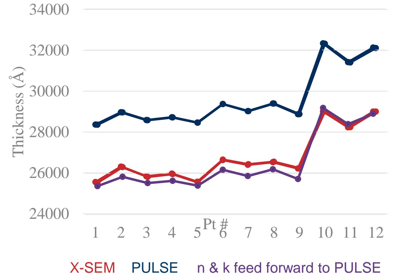
With feed forward, thickness accuracy improved by 10X compared to X-SEM
