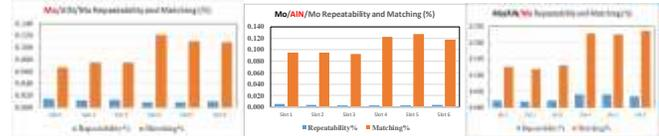
Figure 6. Mo, AlN and Mo dynamic repeatability and tool to tool matching for the tri-layer stack Mo/AlN/Mo.
