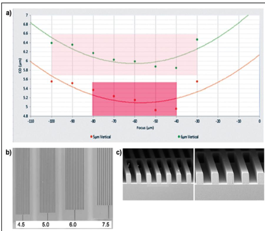
**Figure 6:** a) Bossung plot generated from FEM data showing less than 10% deviation over 40µm DOF for 5µm lines and 70µm DOF for 6µm lines. b) Lower resolution image of 4.5µm, 5µm, 6µm and 7.5µm isolated and dense area line/space arrays. c) Higher resolution cross-sectional images of 5µm and 6µm lines in a 10µm-thick dry resist on copper substrate.
