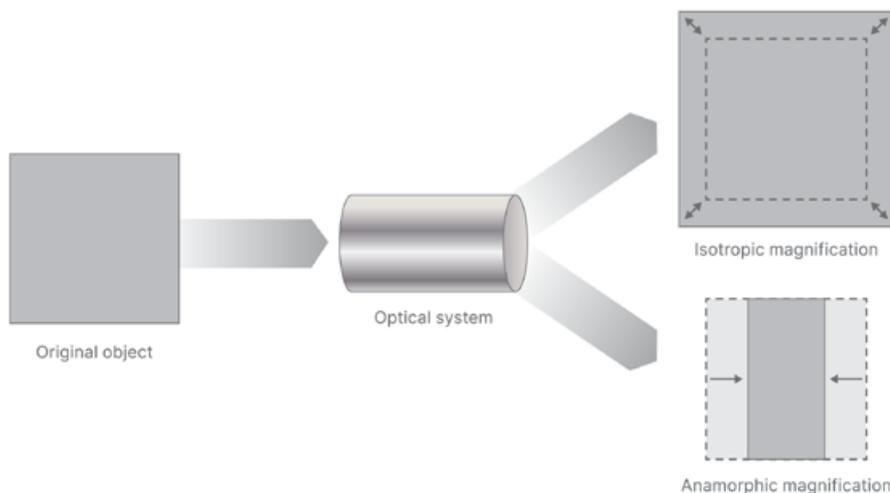
**Figure 4:** Isotropic magnification and anamorphic magnification compensation.
