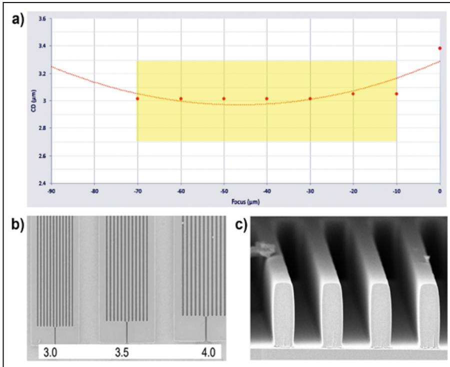
**Figure 5:** a) Bossung plot generated from FEM data showing less than 10% deviation over 60µm DOF; b) Lower resolution image of 3µm, 3.5µm and 4µm isolated and dense area line/space arrays; c) Cross-section image of 3µm lines in 10µm thick dry film resist on copper substrate; the line critical dimension is 3.181µm, and the resist height is 9.873µm in the cross-sectional image.
