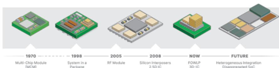
**Figure 1:** Heterogeneous integration enables next-generation device performance gains by combining multiple silicon nodes and designs inside one package. The package size is expected to grow significantly. SOURCE: Cadence
