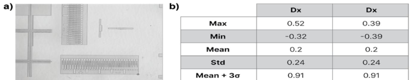
**Figure 9:** A summary of the results of overlay measurements: a) Overlapped verniers included in the pattern were used to measure overlay errors. b) The table summarizes the measured errors.
