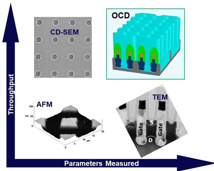
Figure 1. OCD is compared to other CD metrology methods graphed versus throughput and the parameters measured.
