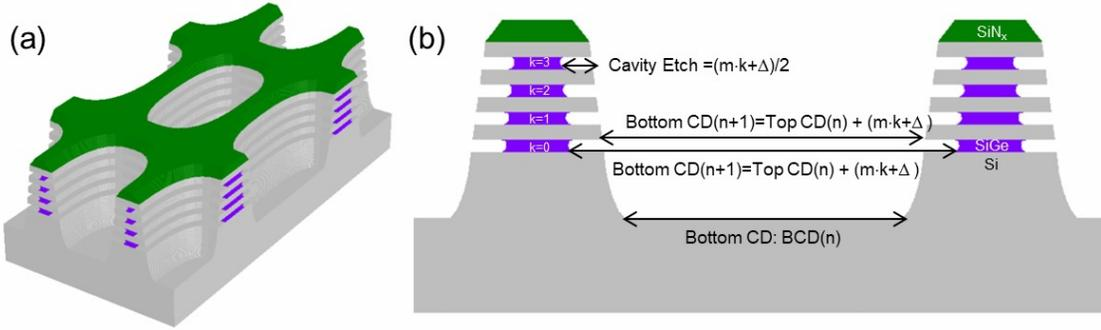
Figure 10. a) Si/SiGe Elliptical Hole Test structure iso view. b) Profile view showing floating CD parameters in the model
