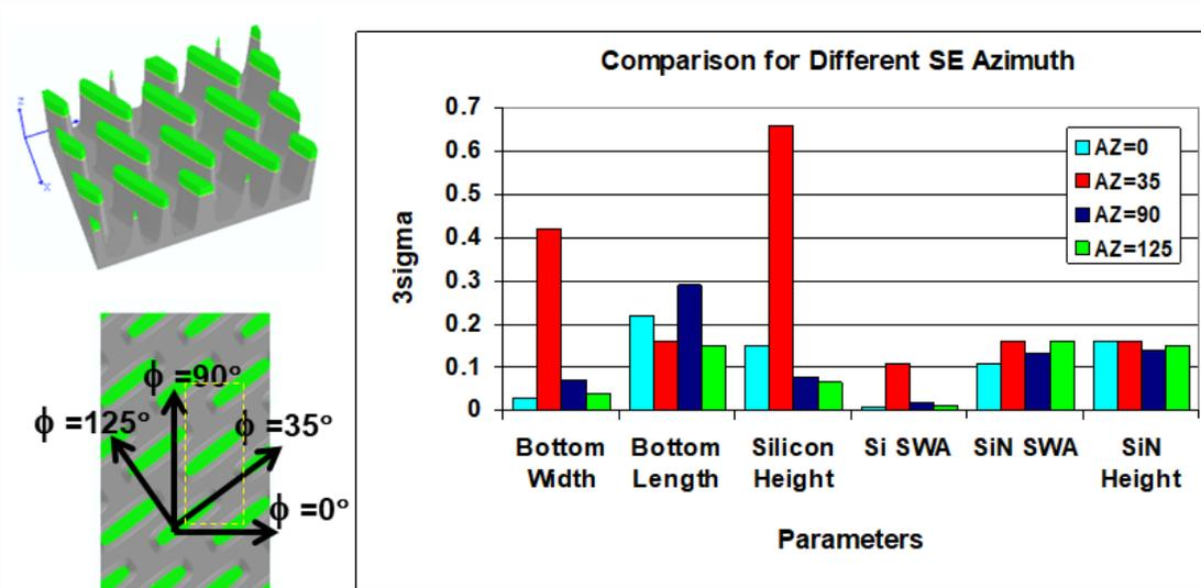
Figure 8. Azimuth Optimization of Rotated STI Island structures using U&SA
