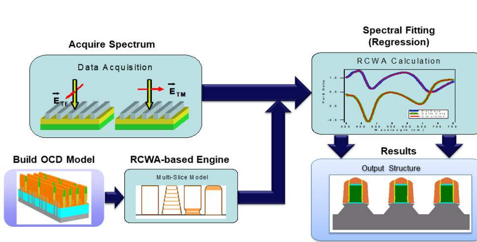
Figure 5. OCD Model Workflow, starting from the left. 1) SE data are acquired. 2) An OCD model is built. 3) An RCWA-based engine calculates the expected response. 4) The unknown sample properties are varied in a spectral fitting process. 5) The results are reported.
