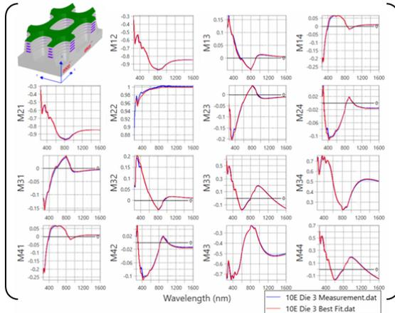
Figure 11. Model fit to Experimental Spectra at 75-degree azimuth angle
