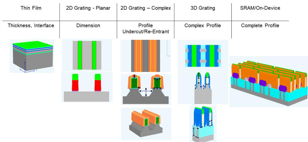
Figure 3. Evolving complexity of Logic devices
