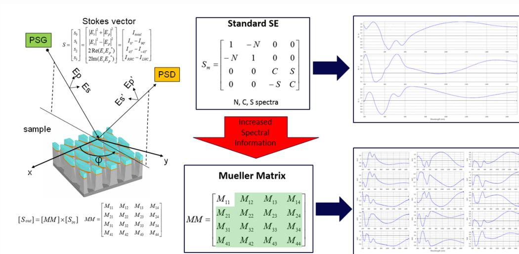
Figure 4. Comparison of "standard" SE and Mueller Matrix SE (MMSE)
