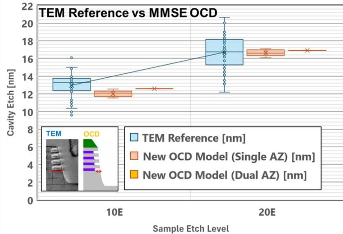
Figure 12. TEM reference vs. OCD results for Cavity Etch
