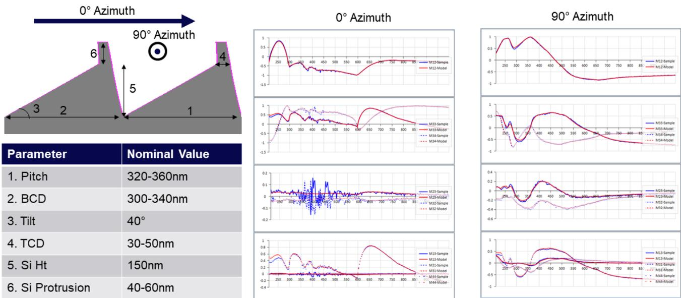
Figure 9. Blazed Surface Relief Grating in Si showing the modeled structure, floating parameters, and model fit at 0 and 90-degree azimuth angles
