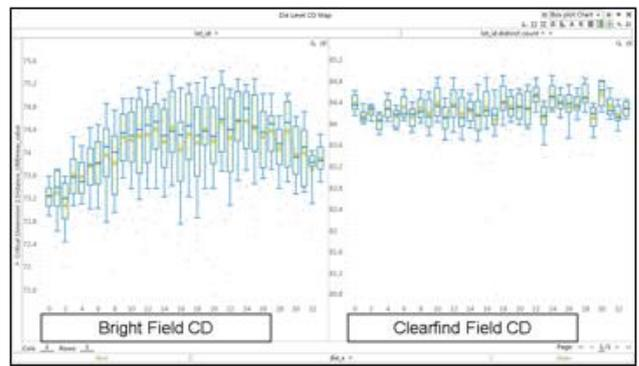
**Figure 7.** Cu pad X dimension CD uniformity comparing BF and Clearfind across the wafer
