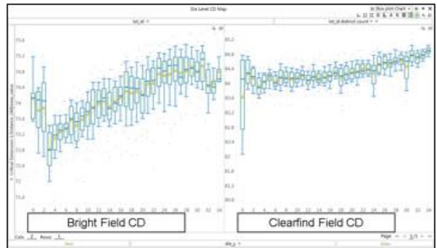
**Figure 8.** Cu pad Y dimension CD uniformity comparing BF and Clearfind across the wafer
