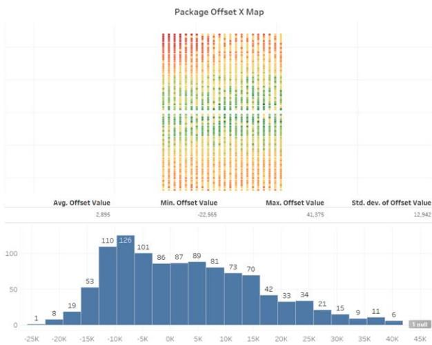
**Figure 16.** Package Position Shift in X as measured on a panel post EMC cure
