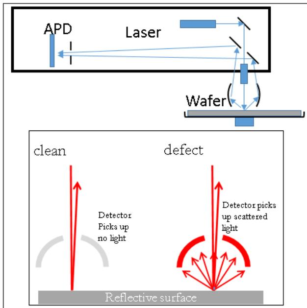
Figure 2. Simplified diagram of LSA particle detection principles.
