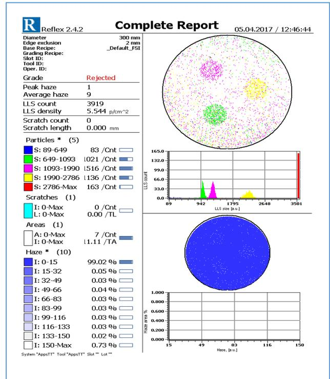
Figure 3. LSA Polystyrene Latex Sphere (PSL) reference defect map
