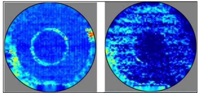
**Figure 14.** Whole wafer CD map comparing Clearfind (right) and Bright Field (left) Cu RDL under etching detection
