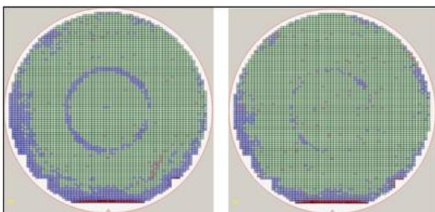
**Figure 13.** 2D Defect map comparing Clearfind (right) and Bright Field (left) maps of Cu RDL under etching defects
