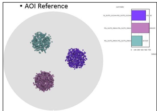
Figure 4. Inspection tool reference map used for capture rate validation against the LSA
