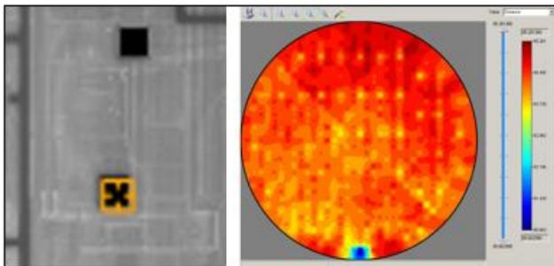
**Figure 6.** Whole wafer Cu pad CD uniformity using method “C”
