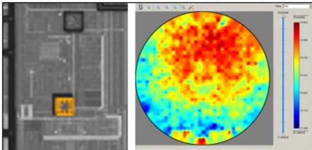
**Figure 5.** Whole Wafer Bright field Cu pad CD uniformity
