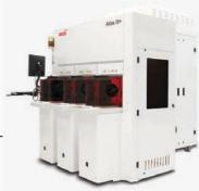
NanoDiffract® and SpectraProbe™. With its unique combination of spectroscopic ellipsometry (SE) with full Mueller Matrix capability and broadband reflectometry (SR), the Atlas III+ provides industry-leading metrology performance while also providing increased productivity on the most demanding devices, both in development and high-volume production.
