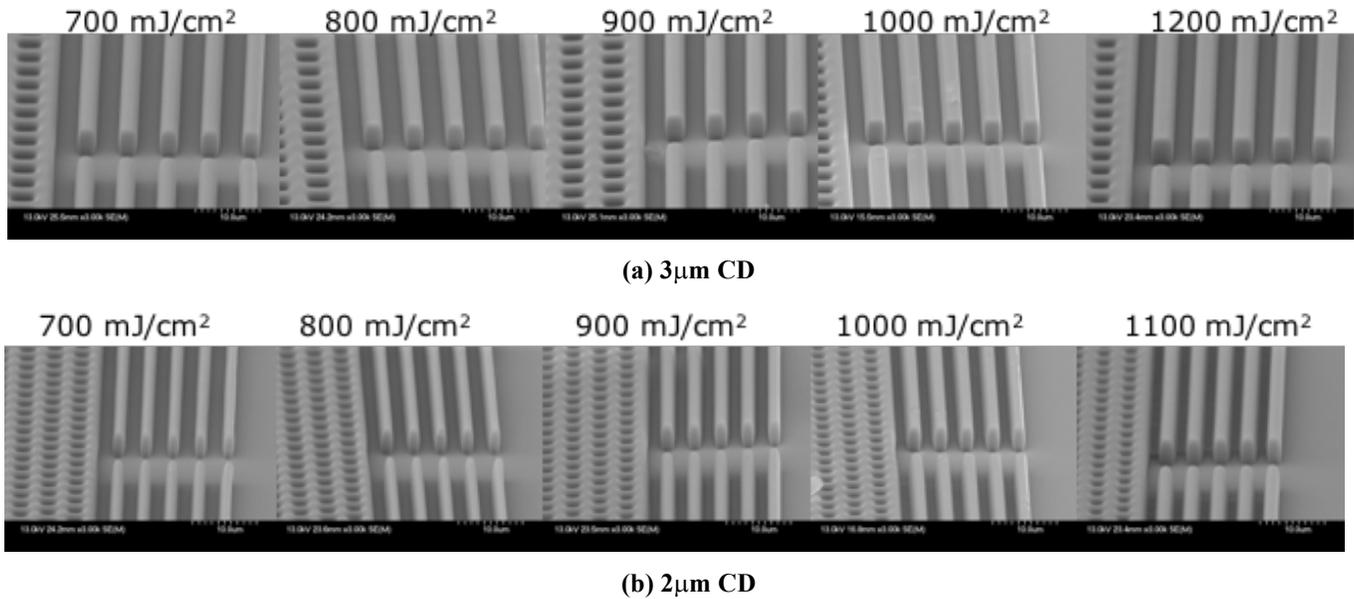
**Figure 6.** (a) Exposure Dose Range of 700-1200 mJ/cm<sup>2</sup> for CD of 3µm, and (b) Exposure Dose Range of 800-1100 mJ/cm<sup>2</sup> for CD of 2µm, both indicating good lithographic definition and CD control
