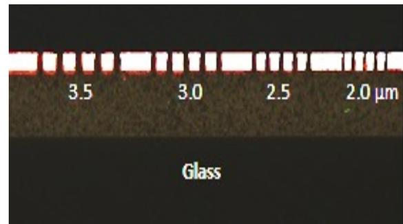
**Figure 8.** Cross-section micrograph of 2µm to 3.5µm embedded copper traces formed in IF4605 dielectric
