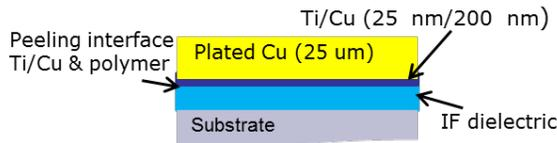
**Figure 3.** Cross-section Schematic of the Peel Strength Test Structure
