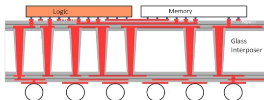
**Figure 1.** Cross-section Schematic of a 2.5D Glass Interposer Package with High Density RDL
