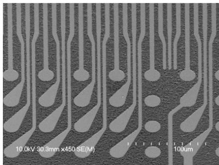
**Figure 9.** Top View of 3.5 $\mu\text{m}$  line width and 2.5 $\mu\text{m}$  space embedded copper structures at 40 $\mu\text{m}$  I/O pitch
