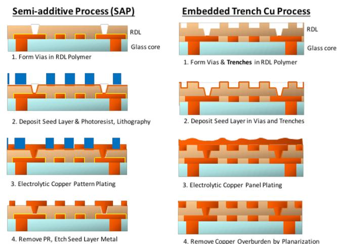
**Figure 2.** Comparison of Process Flows for SAP and Embedded Trench RDL Fabrication
