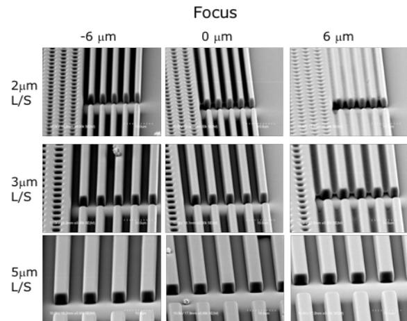
**Figure 7.** SEM micrographs of IF4605 lithography with variation in the focal depth.
