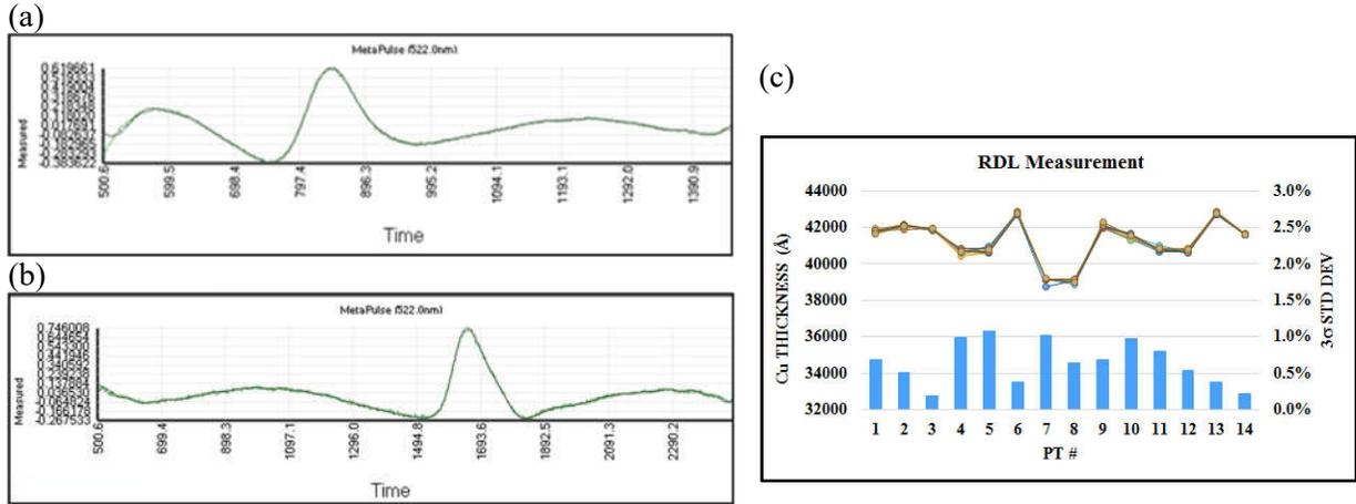
Fig 2. (a) Modeled fit to measured data from a  $2\mu\text{m}$  RDL film. Echo arrives at  $\sim 800$ ps corresponding to a  $2\mu\text{m}$  film. (b) Echo arrival time  $\sim 1600$ ps corresponding to a  $4\mu\text{m}$  RDL film. (c) Cross-wafer thickness variation and repeatability performance shown.
