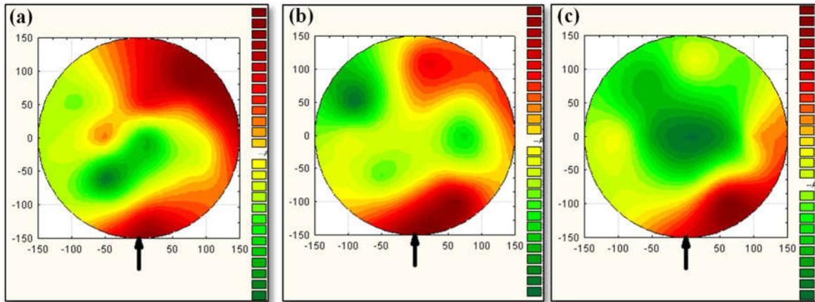
Fig 3. Within wafer uniformity maps of RDL Lines from varying stages of development. (a) 3.5% non-uniformity and (b) 2.3% non-uniformity (c) 2% non-uniformity
