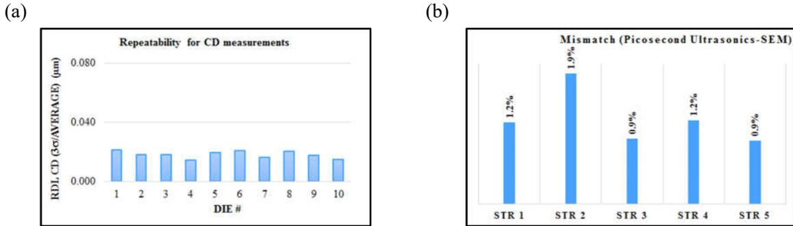
Fig 4(a). Load/unload repeatability measurements of RDL CD from an advanced process. Typical repeatability shown. (b) Structures 1-5 shown in the x-axis represent various RDL structures ( $2\mu m$ - $4\mu m$ ). Mismatch between picosecond ultrasonics and SEM on an average is  $\sim 1.2\%$
