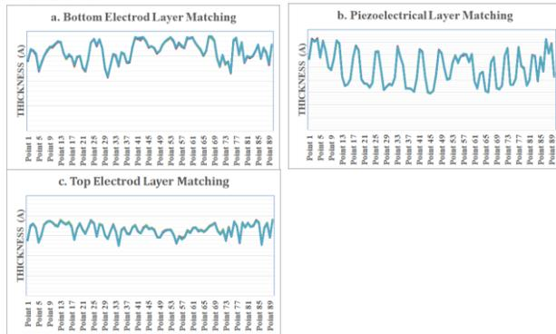
Figure 4. Site level of a). bottom electrode Mo, b). AlN and c). top electrode Mo tool to tool matching for the tri-layer stack Mo/AlN/Mo.
