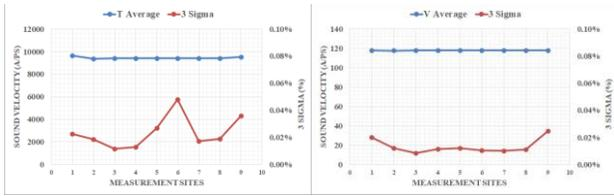
Figure 3a). Example of AlN thickness and repeatability by Picosecond Ultrasonic. 3b). Example of AlN sound velocity and repeatability by Picosecond Ultrasonic.
