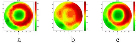
Figure 5. Nearly 400 measurement site maps for a). bottom electrode Mo, b). AlN and c). top electrode Mo for the tri-layer stack Mo/AlN/Mo.
