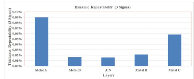
Figure 2. Thickness dynamic repeatability (3σ) for each layer of a five-layer stack metal A/metal B/AlN/metal B/metal C.
