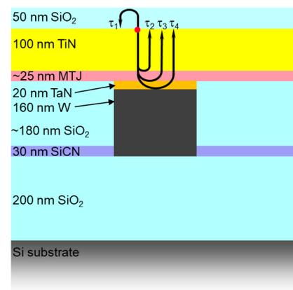
Fig 1. Cross-section of the samples used for picosecond laser acoustic measurements.
