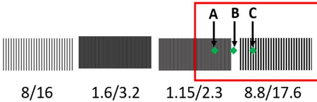
Fig. 2 Target structures used for measurement along with their CD/ pitch (in microns).
