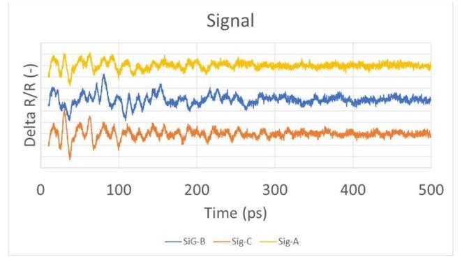
Fig 3. Differential reflectivity signal (after background subtraction) as a function of pump-probe delay plots corresponding to measurements from regions A, B and C.
