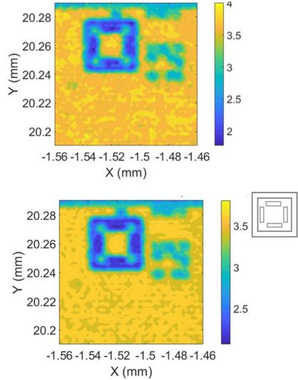
Fig 6a-b. Image of overlay marker under opaque layers using temporal and FFT signal analysis. Inset to the right shows the schematic of the target.
