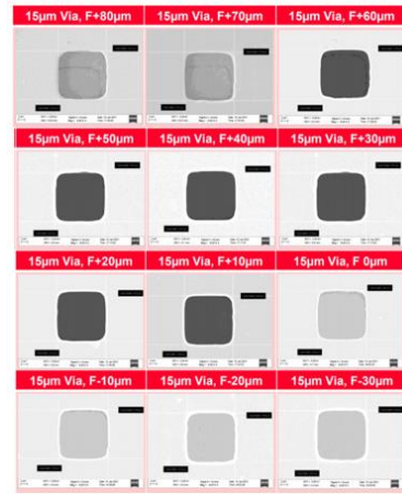
Fig 18. SEM micrographs of 15 \mu\text{m} via imaging results from focus -30 \mu\text{m} to focus + 80 \mu\text{m} .
