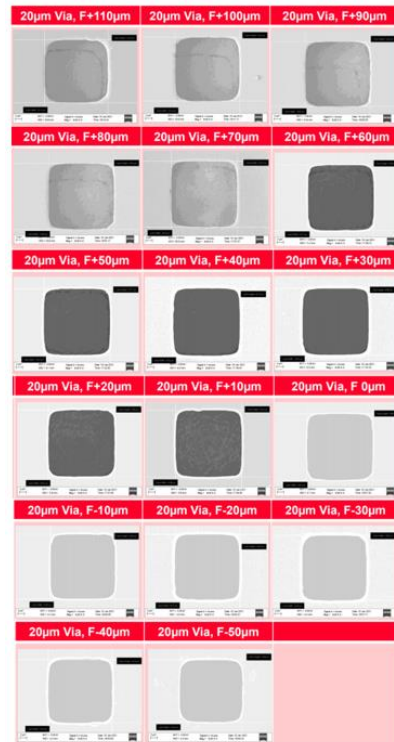
Fig 20. SEM micrographs of 20 \mu\text{m} via imaging results from focus -50 \mu\text{m} to focus +110 \mu\text{m} .
